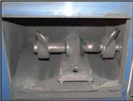
Dust box testing simulates an extremely dusty or dirty environment you might find in industries such as aggregate, mining and cement. The Baldor•Dodge XTS seal showed significantly less lubrication contamination compared to competitor's products.
