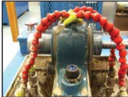
Water and slurry ingress testing simulates operating conditions found in wet environments that would be present in industries such as food processing, lumber and paper.
